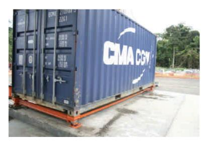
The *Griffith Elder Container Weigher* is purpose designed to weigh industrial containers, whether for check weighing and recording or for monitoring overloads while filling.
