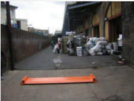
The Ton-Tel™ Portable Weighbridge has been designed to meet the needs of Law Enforcement agencies and other organisations where portability is of prime importance. The platform has a width of 2.5 metres so that a wide range of vehicles can be weighed correctly even though the platform sits on the surface. On some surfaces it is best to hold the platform down to the ground so that it will not move when any vehicle drives onto it.
