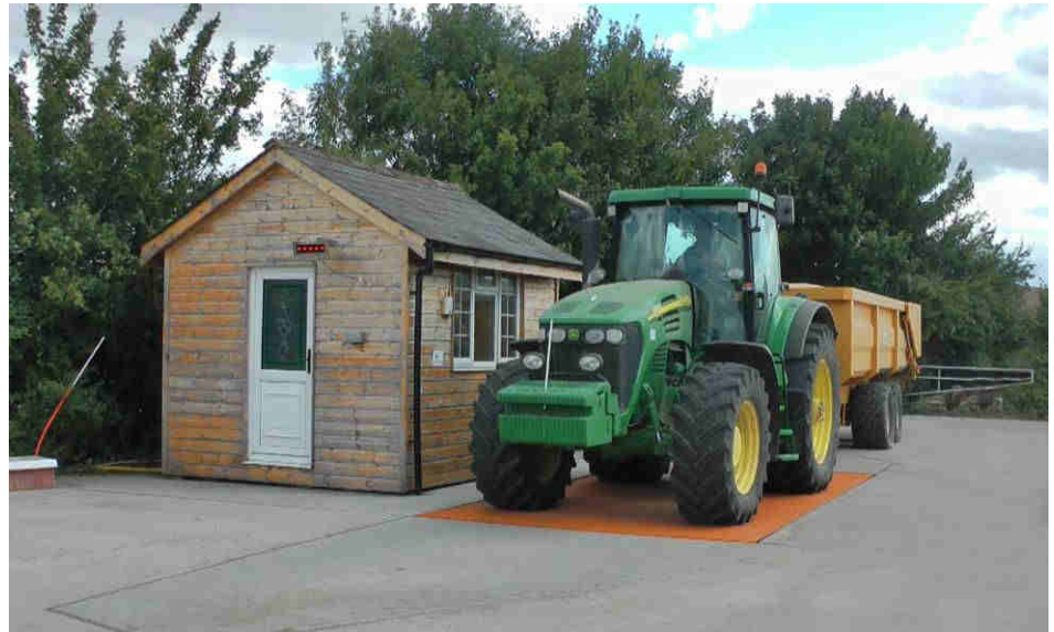
Tractor on 6.0 metre platform
