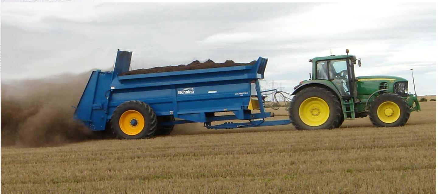
The Griffith Elder *Spreader Monitor* is an automatic weighing system used to monitor and control fertiliser and manure spreaders.
