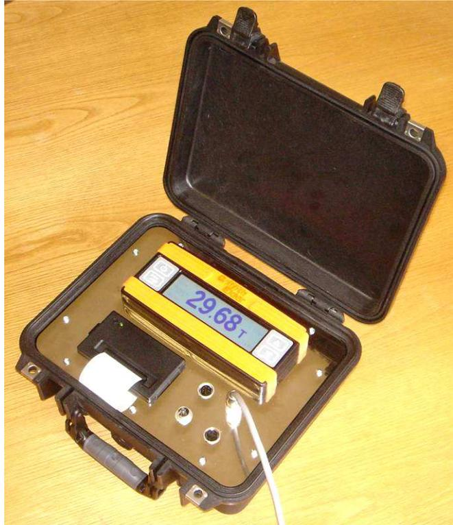
The indicator and printer are built into a tough waterproof suitcase housing for ease of carrying between locations. When the lid is closed the printer is completely waterproof which makes it very suitable for locations with no site hut.
