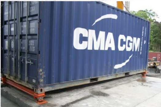
The *Griffith Elder Container Weigher* is purpose designed to weigh industrial containers, whether for check weighing and recording or for monitoring overloads while filling.
