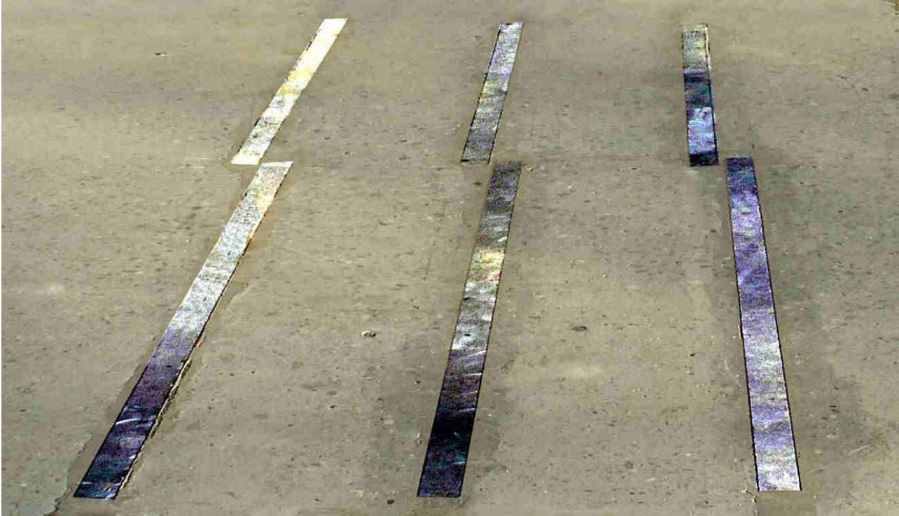
Quartz Weight Sensors installed in a concrete road
