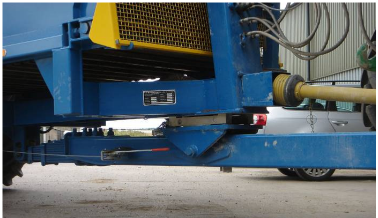
Two 20 tonne Load cells mounted between axle and body Two more Load cells on the drawbar
