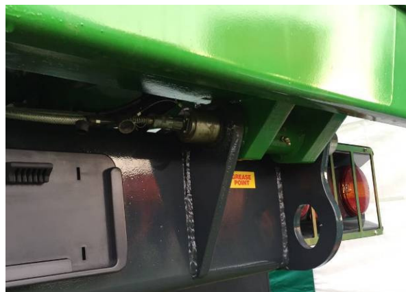
Body pivots on load cell pins
