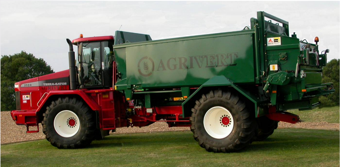
Agchem bodied Terra-Gator manure spreader with 12 tonne shear-beam load cells between body and chassis
