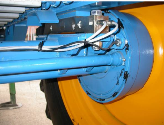
Two 20 tonne Load cells mounted between axle and body Two more Load cells on the drawbar
