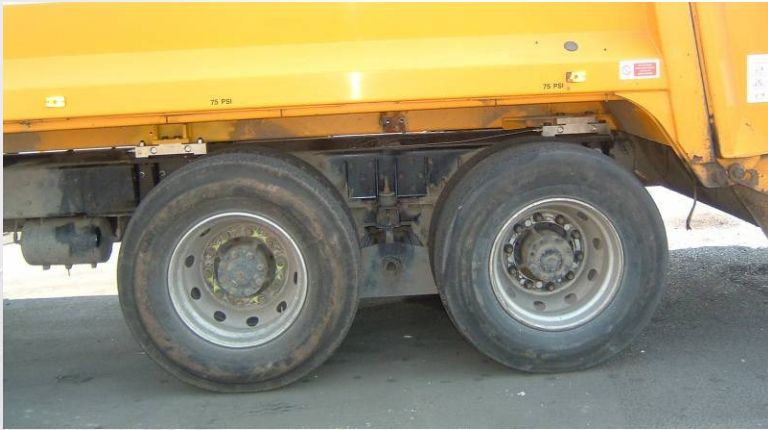
Load Cells mounted between truck chassis and body
