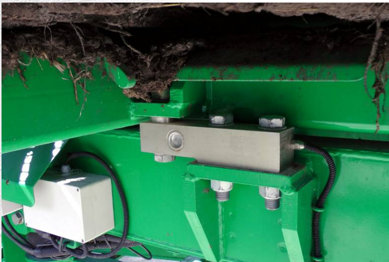
Close-up of 12 tonne shear-beam load cell mounted to the chassis
