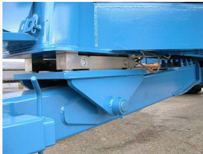
Two 20 tonne Load cells mounted between axle and body Two more Load cells on the drawbar
