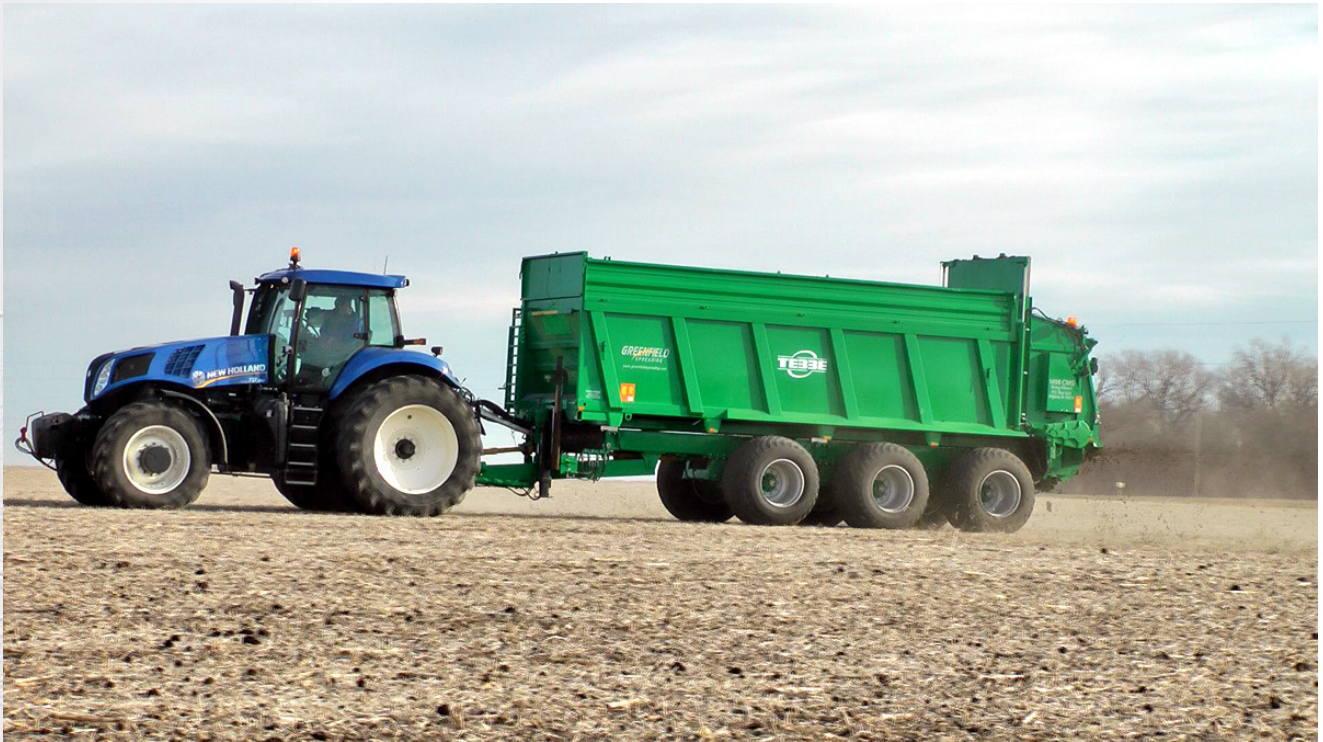
Tebbe 40 tonne spreader with load cells between chassis and body
