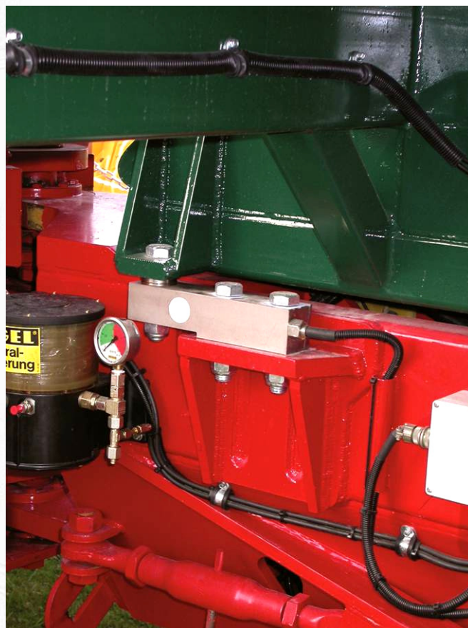
Four 12 tonne shear-beam load cells mounted to the chassis
