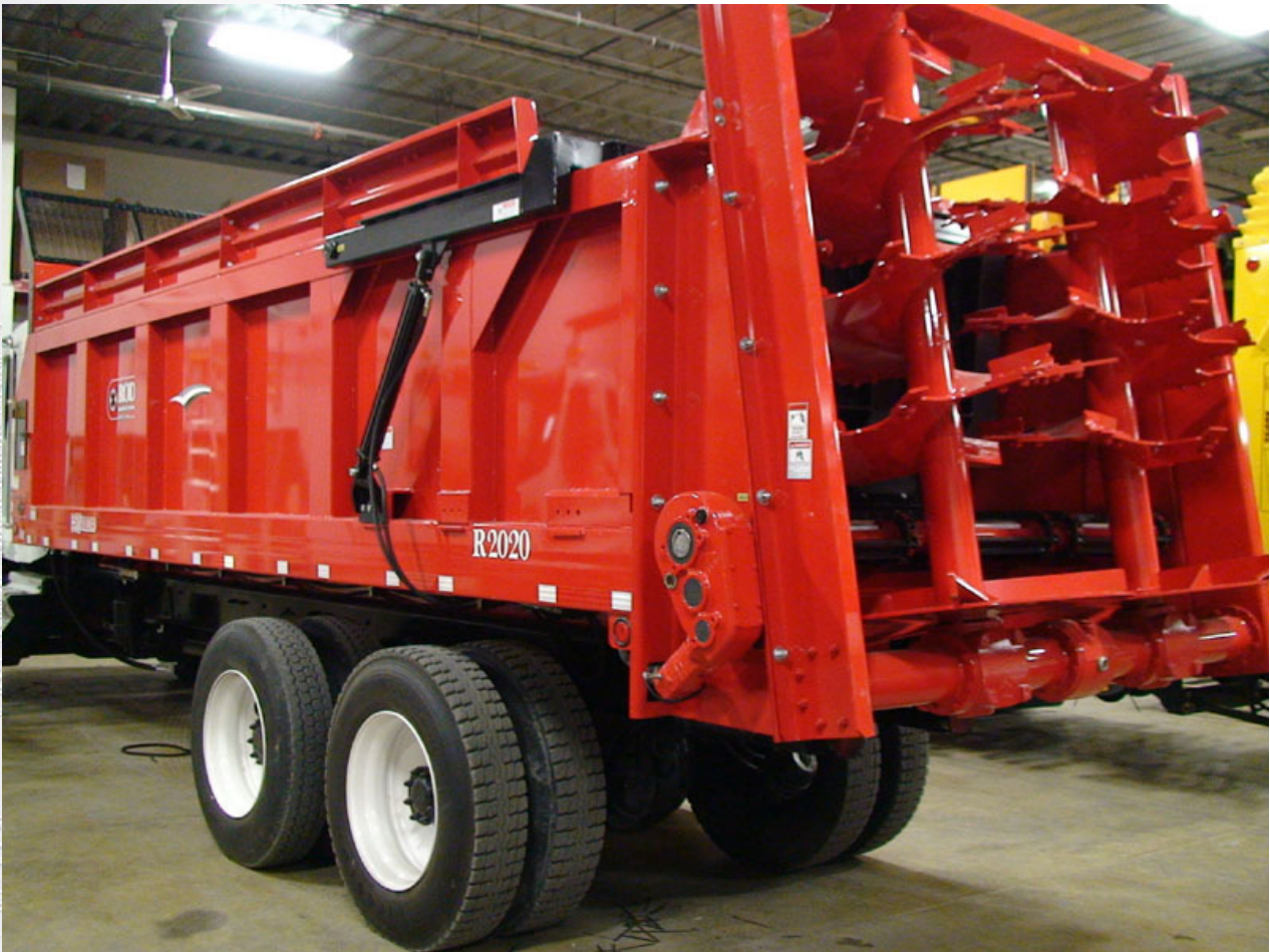
Roda Spreader with double ended shear-beam load cells between body and chassis
