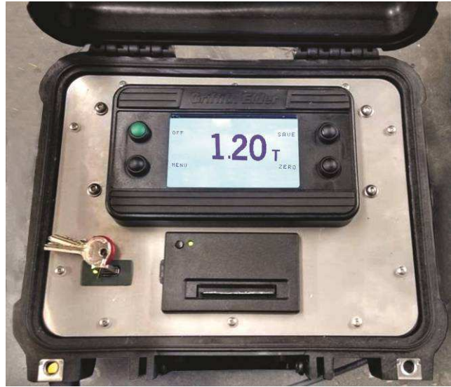
WB6 Indicator with USB Memory, Fob Control and Printer in Waterproof Housing
