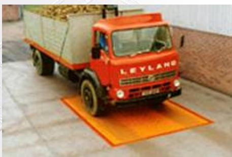
The Griffith Elder range of platform scales are designed to be very robust for continuous industrial use. The all welded steel construction is very durable under harsh conditions.
