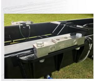
The Griffith Elder *Trailer Weigher* is an accurate weighing system used to measure and record every load carried.
