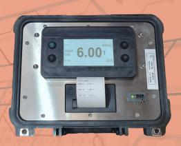
The WB6 indicator and printer stores tare (empty vehicle) weights in its memory, showing, and printing gross, tare and net weights, date, time and ticket number.
